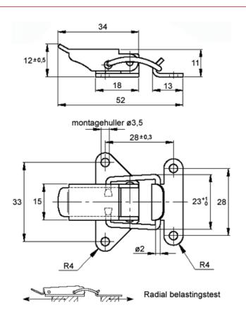
$\begin{array}{l} \text{Max load (N)} &= 550 \\ \text{Ultimate strength (N)} &= 1800 \end{array}$
